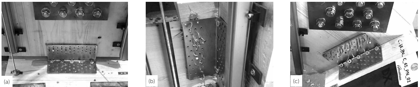
Samples at the end of cyclic tests: tension (a), shear (b) and 45^\circ (c) (partial fastening).
