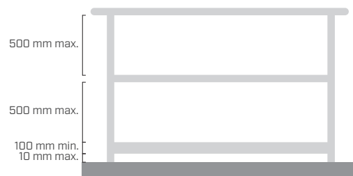
RAILING WITH TOE BOARD
